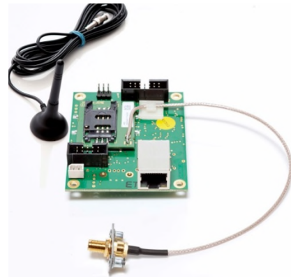
SEXC30REMC+ ETHERNET WEB-SERVER / SNMP AND GSM CONTROL ADAPTER BOARD
