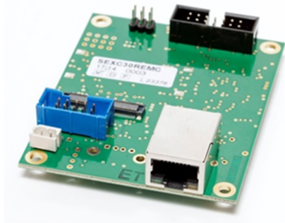
SEXC30REMC ETHERNET WEB-SERVER / SNMP CONTROL ADAPTER BOARD
